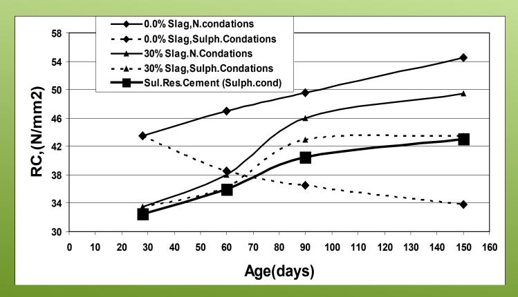
\*the sample with 30% added slag behaves as Anti-sulfate cement and matches its standard properties. As we can observe, it starts with low compressive strengths and it increases by time. Especially long periods of time.
